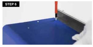
6. Once the UV lamp is installed, reinstall the reflecting tube. It is important to note that the air should first flow through the turbulator before moving in front of the UV lamp.
