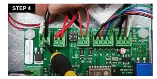
4. After the test is completed, unplug the unit and replace the black wire from the cord in its original position identified "Line".
