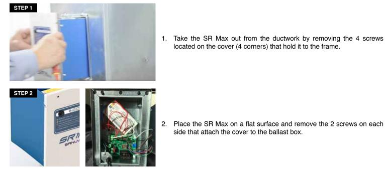
B. Step by Step UV Lamp Continuity Test
