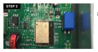
Plug in the SR Max to a power source and turn ON the unit by pressing the power button. In the first 5 seconds from powering the unit ON, click the Reset button once. By doing so, you'll see the status LED turn Blue meaning the airflow detection is activated. By clicking again within 5 seconds, LED will turn White meaning that airflow detection is deactivated.
