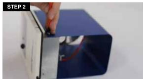
2. Release the reflecting tube by removing the 2 screws on each side to access the lamp.
