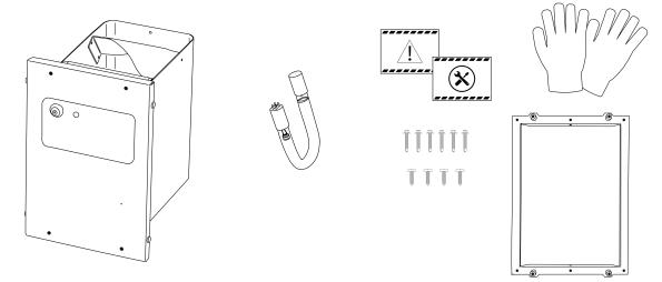
The installation kit includes: a UV caution decal, a maintenance decal, a pair of cotton gloves, metal screws for frame (6), Phillips screws for cover (4) and a frame.
