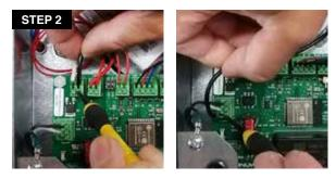
Unplug the ballast black wire from the circuit board. Insert that wire into the connector identified "Bypass".
